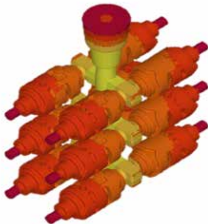
Temperature profile during Investment Casting process
