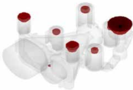
Part shrinkage porosity volume displayed for part shrinkage location
