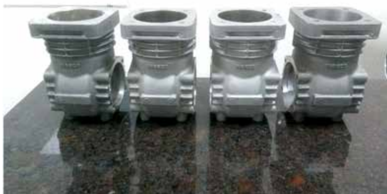
Aluminum alloy crankcase supplied by CSIR-NIIST to WABCO India Limited
